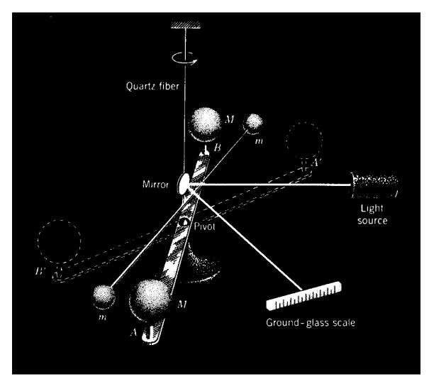
The Cavendish balance, used for experimental verification of Newton's Law of Universal Gravitation. Masses m and m are suspended from a quartz fiber. Masses M and M can rotate on a stationary support. An image of the l amp filaments is reflected by the mirror attached to m and m onto the scale so that any rotation of m and m can be measured.
